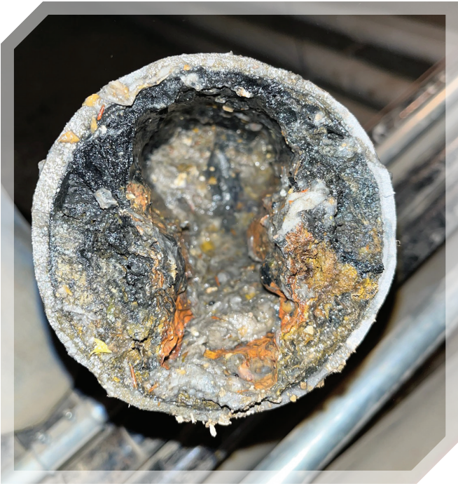
Many of the pipes in the school are originals from 1938 and are corroded beyond further repair. A large portion of the proposal includes replacing the old cast iron pipes with pipes made of modern materials that are designed to reduce corrosion.
